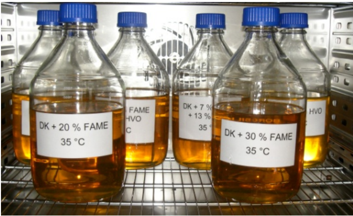
Figure 6 : Test Set-up of the Storage in the Heated Cabinet.
